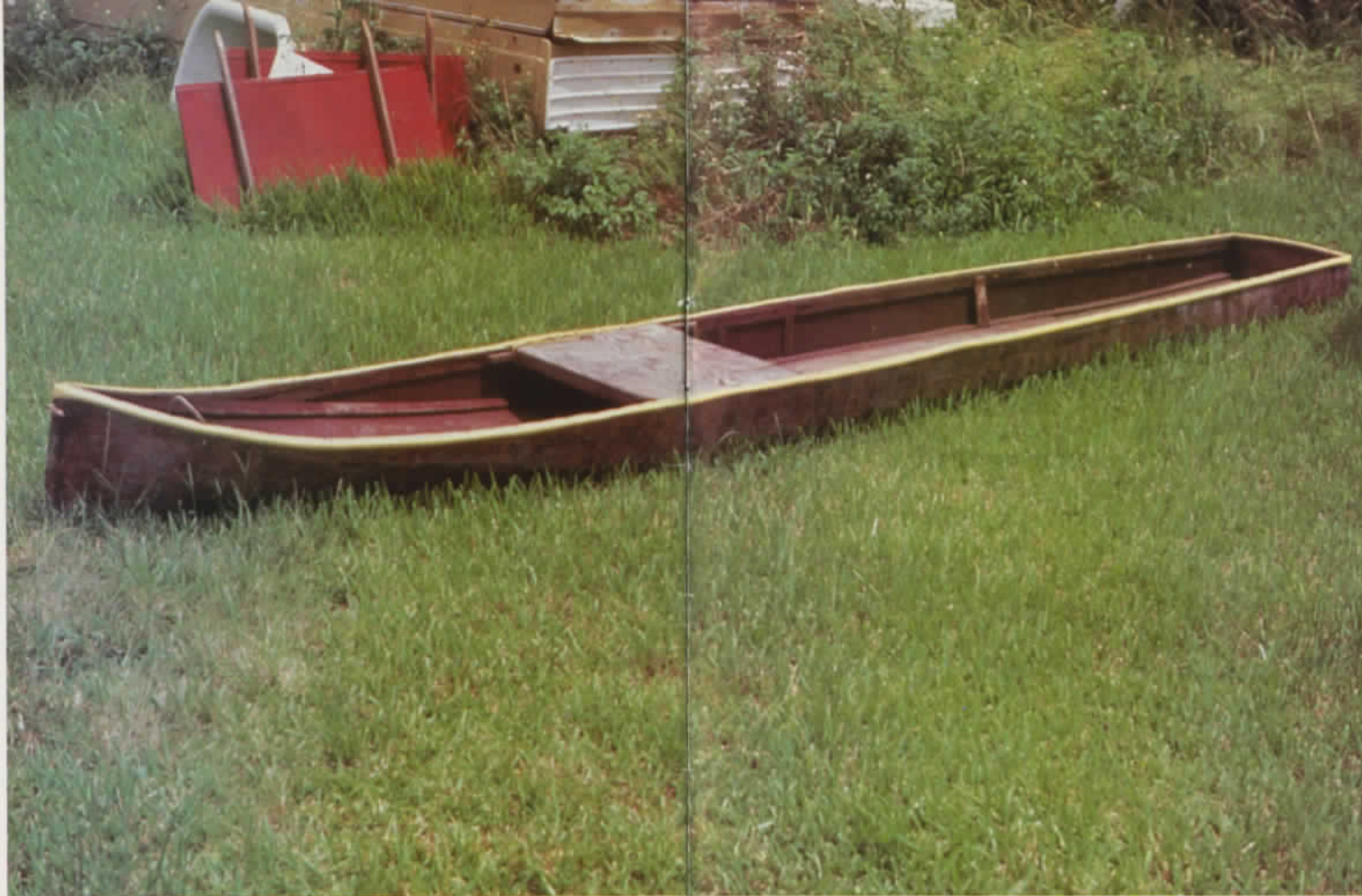
The Everglade skiff's flat bottom and long narrow shape enable it to glide long distances
